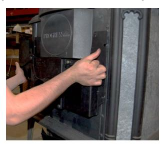
3. Insert eight 1/4-20 hex head bolts & washers into the bolt holes on the stove. Four of the bolts will be the new bolts included with the assembly (5/8"); four of them will be re-used from the old damper. Refer to the diagram below to see which bolts are the NEW bolts. (Shown in the picture below).
