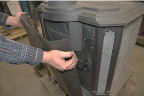
2. Remove the two spacers and 3.75" studs from the rear of the stove under the flue collar.
