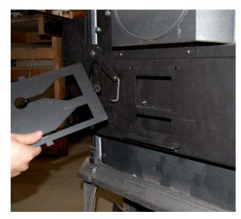
5. Fasten two of the supplied 1/4-20" washers and the two 1/4-20" nuts removed in part 1, step 3 to the studs that protrude through the back of the new air damper. You'll need a wrench to reach the studs on the inside of the damper (see photos below).
