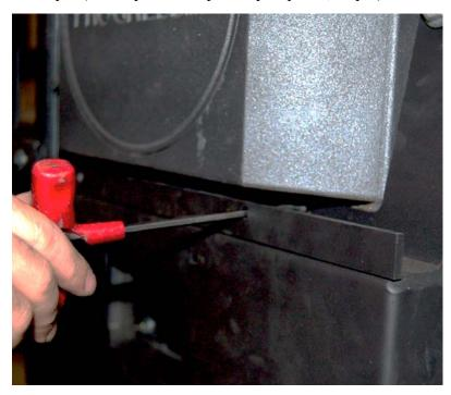
7. Replace the air damper plate, top and bottom retainer plates, and the outside air adapter. Reinstall and tighten the four bolts on the outside air adapter to fasten the assembly back together.
