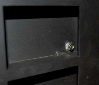
6. Use the guide holes at the top of the air damper to fully tighten the button head allen bolts at the top of the air damper (Initially inserted partially in part 1, step 5).
